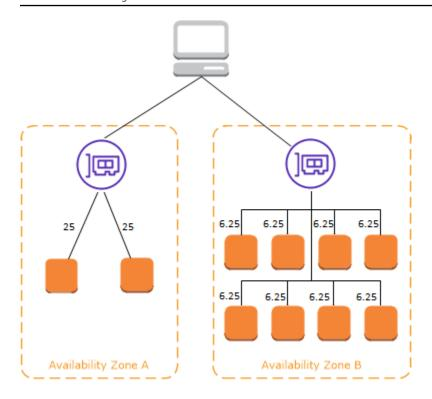
With Application Load Balancers, cross-zone load balancing is always enabled at the load balancer level. At the target group level, cross-zone load balancing can be disabled. For more information, see Turn off cross-zone load balancing in the *User Guide for Application Load Balancers*.
