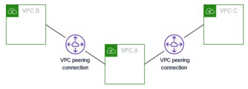
VPC B and VPC C can't send traffic directly to each other through a VPC A, because VPC peering does not support transitive peering relationships. You can create a VPC peering connection
