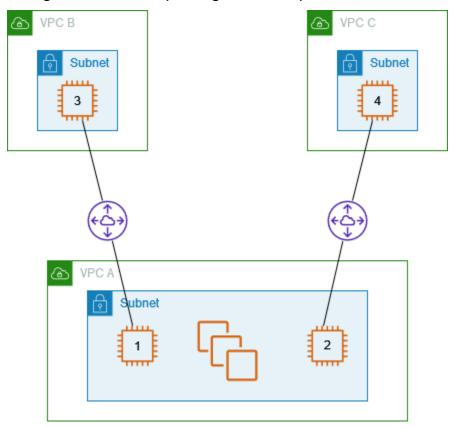
Each VPC route table points to the relevant VPC peering connection to access a single IP address (and therefore a specific instance) in the peer VPC.
