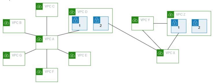
The route tables for VPCs B, C, E, F, and G point to the relevant peering connections to access the full CIDR block for VPC A, and the VPC A route table points to the relevant peering connections for VPCs B, C, E, F, and G to access their full CIDR blocks. For peering connection pcx-aaaadddd, the VPC A route table routes traffic only to subnet 1 in VPC D and the subnet 1 route table in VPC D points to the full CIDR block of VPC A.
