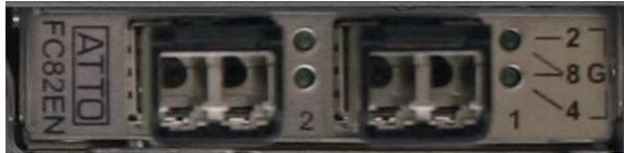
**SFP+ Ports for Fibre Channel**
