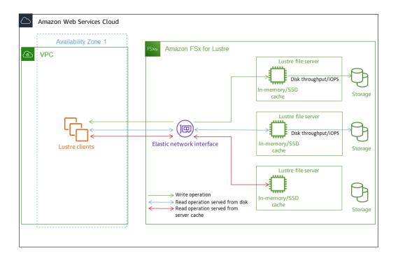
When you read data that is stored on the file server's in-memory or SSD cache, file system performance is determined by the network throughput. When you write data to your file system, or when you read data that isn't stored on the in-memory cache, file system performance is determined by the lower of the network throughput and disk throughput.
