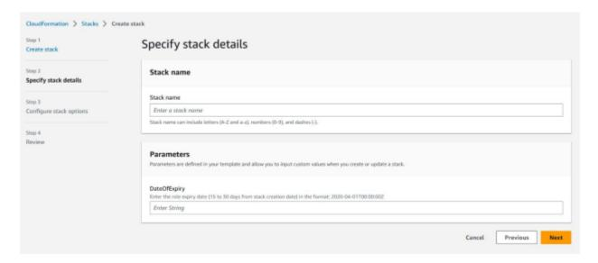
4. Enter the stack name "ams-onboarding-role" in the Stack Name field. Enter a DateOfExpiry using the format "YYYY-MM-DDT00:00:00Z" (30 days from the current date is recommended). Continue scrolling down and selecting next until you reach this page:
