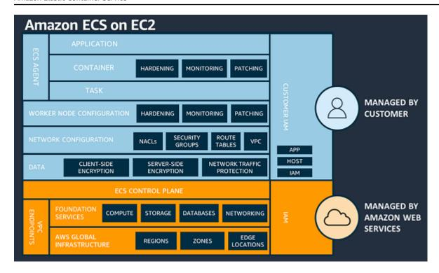
With respect to infrastructure security, AWS assumes more responsibility for AWS Fargate resources than it does for other self-managed instances. With Fargate, AWS manages the security of the underlying instance in the cloud and the runtime that's used to run your tasks. Fargate also automatically scales your infrastructure on your behalf.
