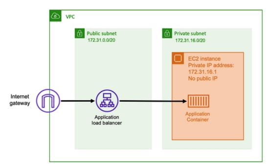
With this architecture, you create an Application Load Balancer in a public subnet so that it has a public IP address and can receive inbound connections from the internet. When the Application Load Balancer receives an inbound connection, or more specifically an HTTP request, it opens a connection to the application using its private IP address. Then, it forwards the request over the internal connection.
