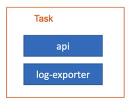
We don't recommend that you use multiple containers in a single task definition for grouping different types of application container. The purpose of having multiple containers in a single task definition is so that you can deploy sidecars, small addon containers that enhance a single type of container. A sidecar might help with logging and observability, traffic routing, or other addon features.
