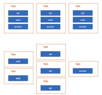
If you group multiple types of application container together in the same task definition, you can't independently scale those containers. For example, it's unlikely that both a website and an API require scaling out at the same rate. As traffic increases, there will be a different number of web
