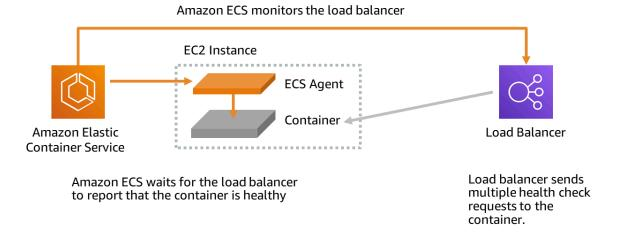
Two Elastic Load Balancing health check parameters affect deployment speed:
