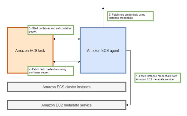
You can manually retrieve the temporary role credentials from inside a container by appending the environment variable to the IP address of the Amazon ECS container agent and running the curl command on the resulting string.
