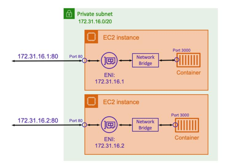
With a static port mapping, you can explicitly define which host port you want to map to a container port. Using the example above, port 80 on the host is being mapped to port 3000 on
