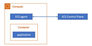
If the application process crashes or ends, the container also ends. If the application must be restarted on crash, let Amazon ECS manage the application restart externally. The Amazon ECS agent reports to the Amazon ECS control plane that the application container crashed. Then, the control plane determines whether to launch a replacement container, and if so where to launch it. The replacement container may be placed onto the same host, or onto a different host in the cluster.
