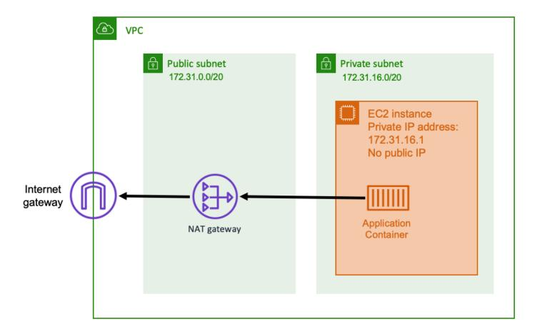
By using a private subnet and a NAT gateway, you can run your containerized application on a host that's in a private subnet. As such, this host has a private IP address that's routable inside your VPC, but isn't routable from the internet. This means that other hosts inside the VPC can make connections to the host using its private IP address, but other hosts on the internet can't make any inbound communications to the host.
