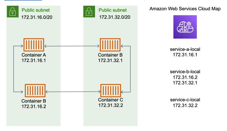
In the preceding diagram, there are three services. serviceA has one container and communicates with serviceB, which has two containers. serviceB must also communicate with serviceC, which has one container. Each container in all three of these services can use the internal DNS names from AWS Cloud Map to find the internal IP addresses of a container from the downstream service that it needs to communicate to.
