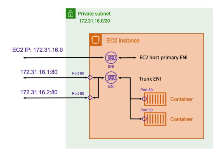
When using ENI trunking, two ENI attachments are used by default. The first is the primary ENI of the instance, which is used for any host level processes. The second is the trunk ENI, which Amazon ECS creates. This feature is only supported on specific Amazon EC2 instance types.
