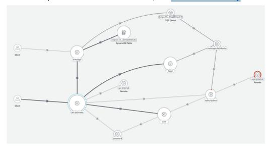
You can also explore AWS X-Ray graphs of how your services network with each other. Or, use them to explore aggregate statistics about how each service-to-service link is performing. Last, you can dive deeper into any specific transaction to see how segments representing network calls are associated with that particular transaction.
