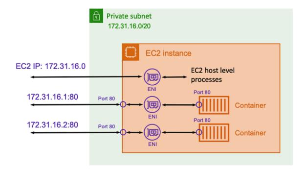
In the preceding example, the Amazon EC2 instance is assigned to an ENI. The ENI represents the IP address of the EC2 instance used for network communications at the host level. Each task also has
