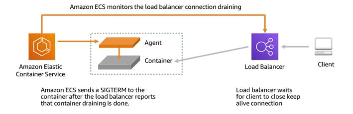
The amount of time that the load balancer waits is the deregistration delay. You can configure the following load balancer setting to speed up your deployments.
