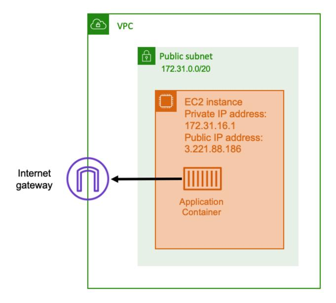
By using a public subnet that has a route to an internet gateway, your containerized application can run on a host inside a VPC on a public subnet. The host that runs your container is assigned a public IP address. This public IP address is routable from the internet. For more information, see <a href="Internet gateways">Internet gateways</a> in the Amazon VPC User Guide.
