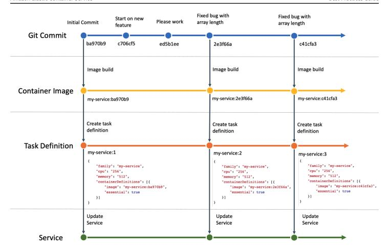
Make sure that there's a one-to-one mapping between a version of application code, a container image tag, and a task definition revision. A typical release process involves a git commit that gets turned into a container image that's tagged with the git commit SHA. Then, that container image tag gets its own Amazon ECS task definition revision. Last, the Amazon ECS service is updated to tell it to deploy the new task definition revision.
