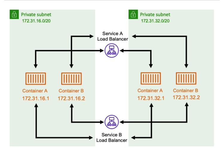
The load balancer maintains high availability by deploying redundant resources into each subnet. When a container from serviceA needs to communicate with a container from serviceB, it opens a connection to the load balancer. The load balancer then opens a connection to a container from service B. The load balancer serves as a centralized place for managing all connections between each service.
