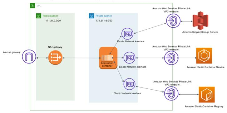
The following are some of the common VPC endpoints that are used with the Amazon ECS service.
