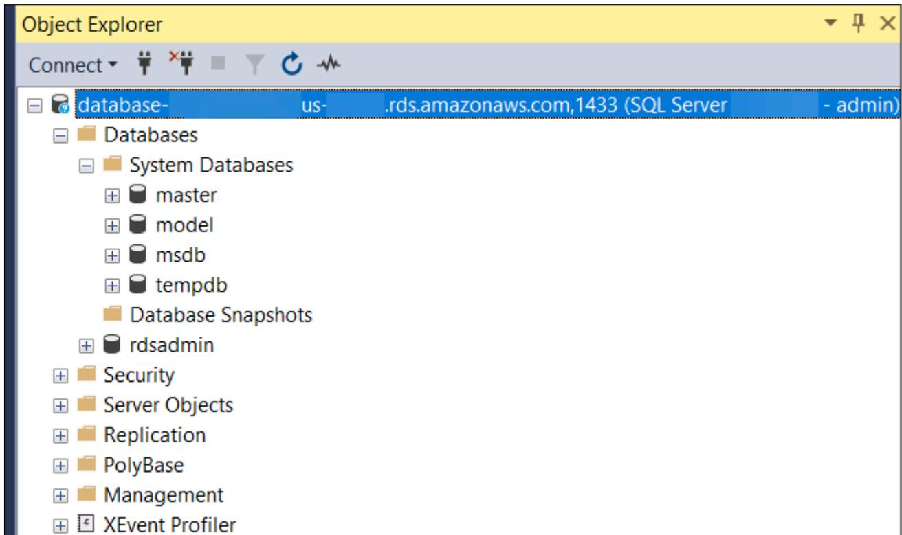
Your SQL Server DB instance also comes with a database named `rdsadmin`. Amazon RDS uses this database to store the objects that it uses to manage your database. The `rdsadmin` database also includes stored procedures that you can run to perform advanced tasks.
