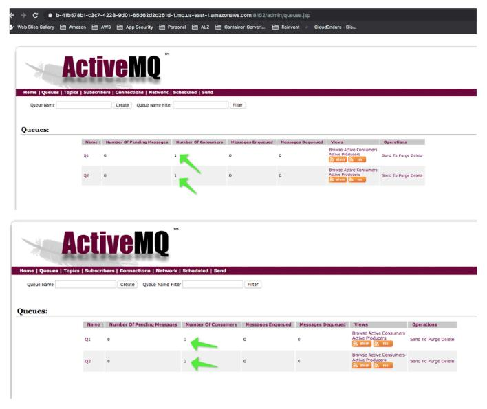
2. Both queues are now available to both brokers, producers can send messages to any broker, and subscribers can receive messages from any broker. For *JMS 1.1* compliant applications, change the endpoint URL to an ActiveMQ failover URL.
