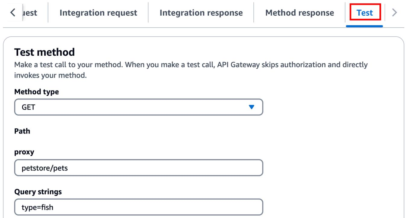
The screenshot shows the 'Test' tab in the Amazon API Gateway console. The 'Method type' is set to 'GET'. The 'Path' is '/petstore/pets'. The 'Query strings' are 'type=fish'. The 'Test' button is highlighted with a red box.
