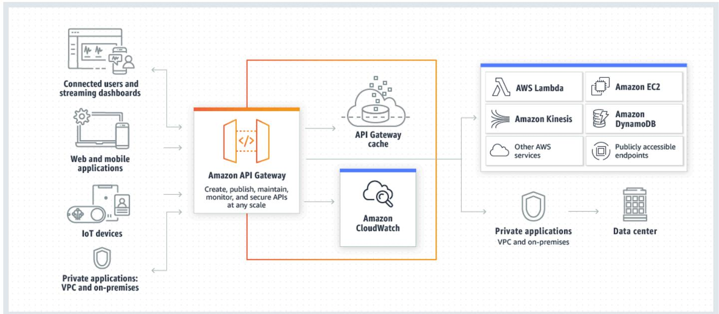
This diagram illustrates how the APIs you build in Amazon API Gateway provide you or your developer customers with an integrated and consistent developer experience for building AWS serverless applications. API Gateway handles all the tasks involved in accepting and processing up to hundreds of thousands of concurrent API calls. These tasks include traffic management, authorization and access control, monitoring, and API version management.
