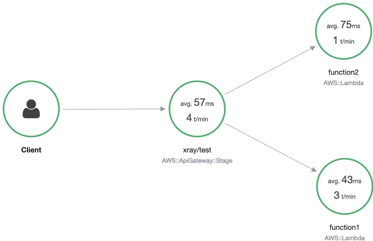
From the service map, you can zoom in to see a trace view of your API stage. The trace will display in-depth information regarding your API, represented as segments and subsegments. For example, the trace for the service map shown above would include segments for the Lambda service and Lambda function. For more information, see [AWS Lambda and AWS X-Ray](#).
