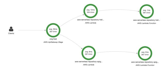
From the service map, you can zoom in to see a trace view of your API stage. The trace will display in-depth information regarding your API, represented as segments and subsegments. For example, the trace for the service map shown above would include segments for the Lambda service and Lambda function. For more information, see Lambda as an AWS X-Ray Trace.
