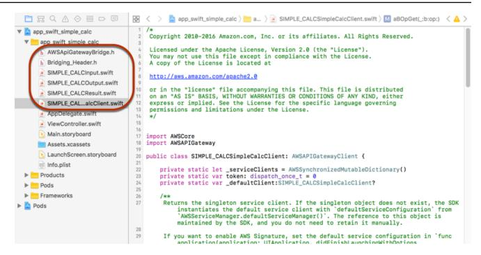
f. To enable calling the Objective-C libraries of the AWS Mobile SDK from your Swift code project, set the Bridging\_Header.h file path on the **Objective-C Bridging Header** property under the **Swift Compiler - General** setting of your Xcode project configuration:
