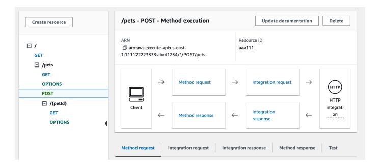
The resulting **Method execution** pane presents a logical view of the chosen (POST /pets) method's structure and behaviors.
