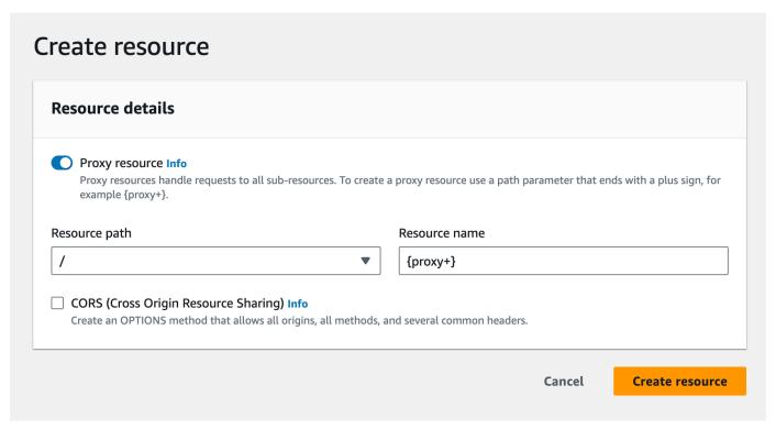
In this step, you integrate the ANY method with a backend HTTP endpoint, using a proxy integration. In a proxy integration, API Gateway passes the client-submitted method request to the backend with no intervention from API Gateway.
