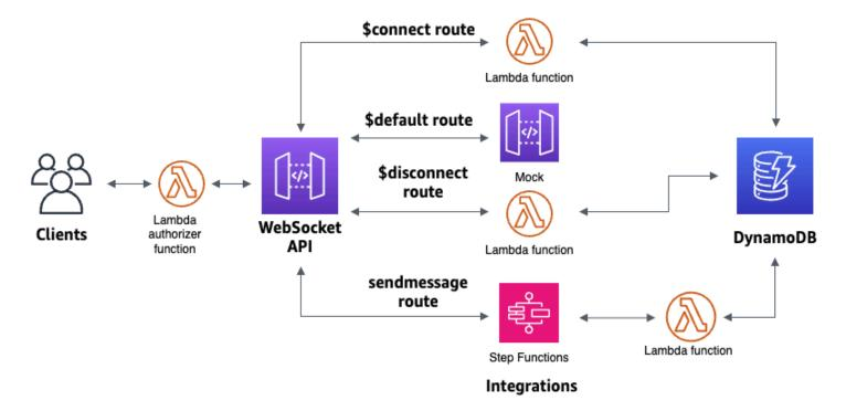
After you create your resources using a AWS CloudFormation template, you'll use the API Gateway console to create a WebSocket API that integrates with your AWS resources. You'll attach a Lambda authorizer to your API and create an AWS service integration with Step Functions to start a state machine execution. The Step Functions state machine will invoke a Lambda function that sends a message to all connected clients.
