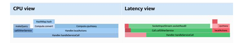
The callOtherService function appears smaller in the **CPU** view because it's not showing the time when the thread was in a waiting state. In the **Latency view**, we still see the part where the CPU was active (in red), but we also see when the threads were waiting (in green).
