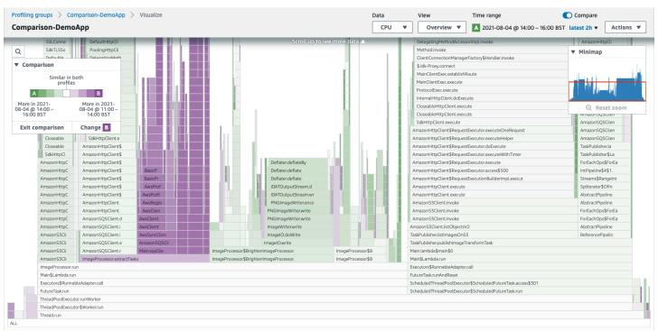
In this example, the two time ranges are A (green) and B (purple). The visualization allows you to pinpoint the areas in darker violet that indicate the function took more time in time range B. Similarly, the darker green indicates functions spending more time in time range A. The more faded sections of the visualization indicate a similar amount of time was taken by the function in both time ranges.
