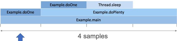
As we collect more samples, the functions in which threads spend a lot of time appear wider in the visualization.
