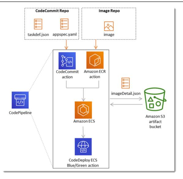
The imageDetail.json file provides the image URI. It must be constructed with the following key-value pair.
