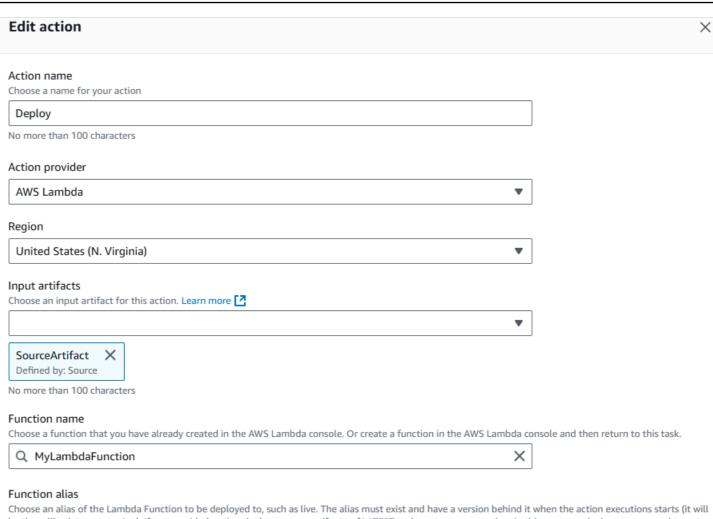
Choose an alias of the Lambda Function to be deployed to, such as live. The alias must exist and have a version behind it when the action executions starts (it will be the rollback target version). If not provided, action deploys source artifact to \$LATEST and creates a new version. In this use case, deploy strategy and target version options are not available.
