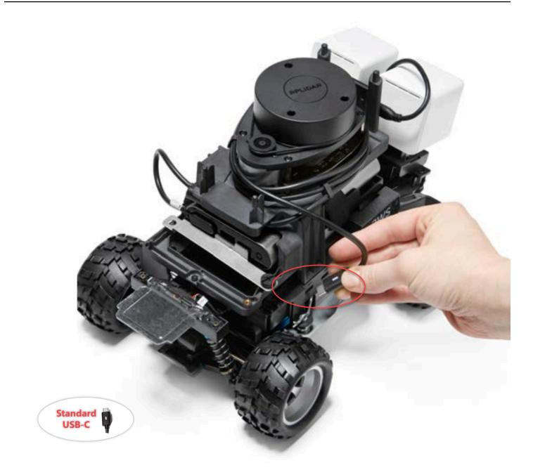
5. Place the Evo shell on your AWS DeepRacer vehicle and fasten it with pins to test the fit. When the shell fits correctly, the LiDAR sensor is fully visible through the cutout in the shell, and you have access to the pin holes on the top of the stanchions. Remove the shell and adjust your cable as necessary.
