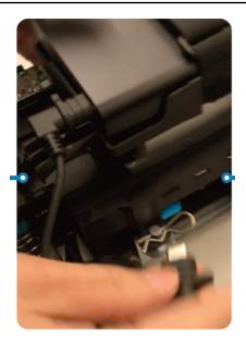
2. Attach the AC power cord and the USB-C cable to the computer module power adapter (A). Plug the power cord to a power outlet (C) and plug the USB-C cable the vehicle's computer module power port (B).
