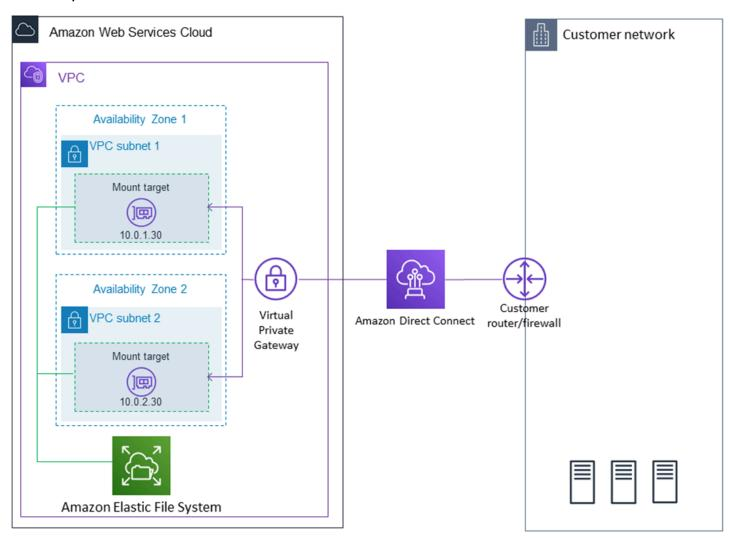
For more information about how to use amazon-efs-utils with AWS Direct Connect and VPN to mount Amazon EFS file systems onto on-premises Linux clients, see <u>Walkthrough: Create and</u> mount a file system on-premises with AWS Direct Connect and VPN.
