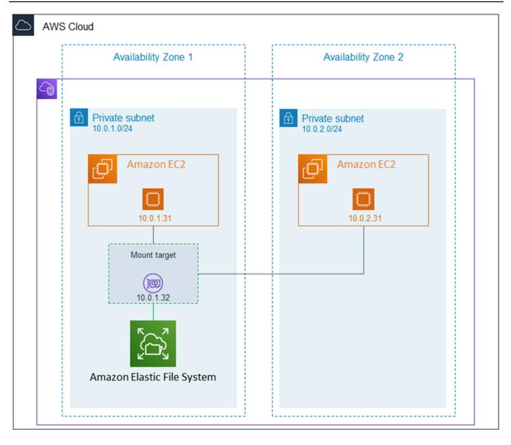
The mount target security group acts as a virtual firewall that controls the traffic. For example, it determines which clients can access the file system. This section explains the following:
