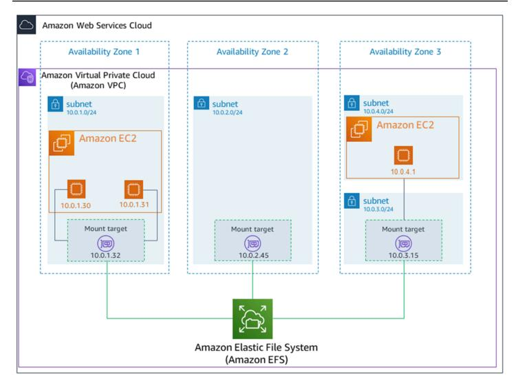
The following diagram shows a One Zone file system, with a single mount target created in the same Availability Zone as the file system. Accessing the file system by using the EC2 instance in the us-west2c Availability Zone incurs data access charges because it is located in a different Availability Zone than the mount target.
