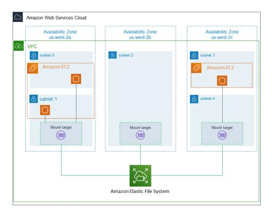
The illustration shows three EC2 instances launched in different VPC subnets accessing an Amazon EFS file system. The illustration also shows one mount target in each of the Availability Zones (regardless of the number of subnets in each Availability Zone).
