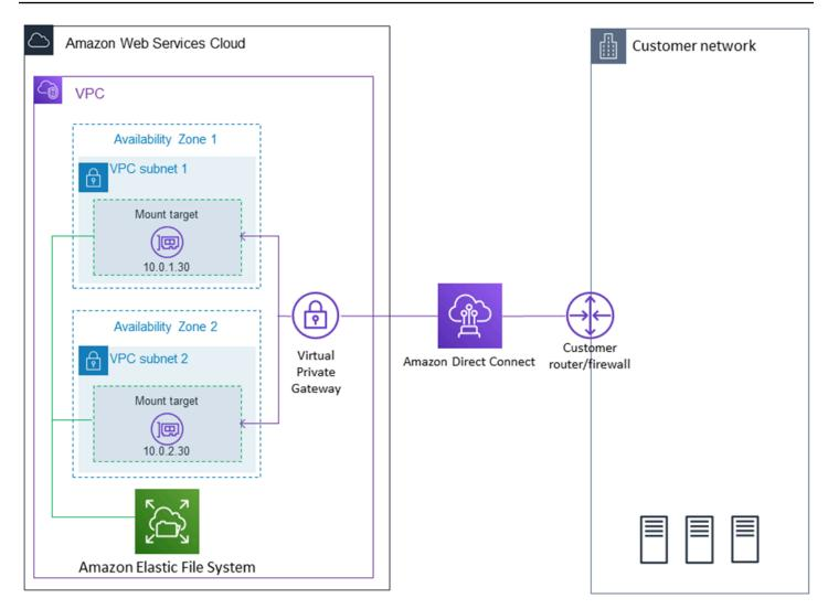
You can use any mount target in your VPC if you can reach that mount target's subnet by using an AWS Direct Connect connection between your on-premises server and VPC. To access Amazon EFS from an on-premises server, add a rule to your mount target security group to allow inbound traffic to the NFS port (2049) from your on-premises server. For more information, including detailed procedures, see <u>Walkthrough: Create and mount a file system on-premises with AWS</u> Direct Connect and VPN.
