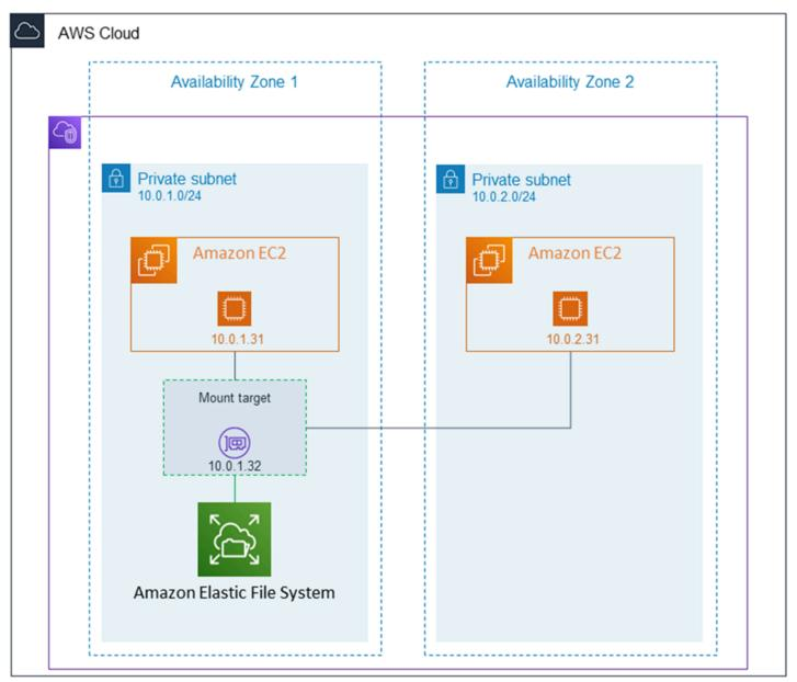
In this illustration, the VPC has two Availability Zones, each with one subnet. Because the file system type is One Zone, it can only have a single mount target. For better performance and cost, we recommend that you access the file system from a mount target in the same Availability Zone as the EC2 instance that you're mounting it on.
