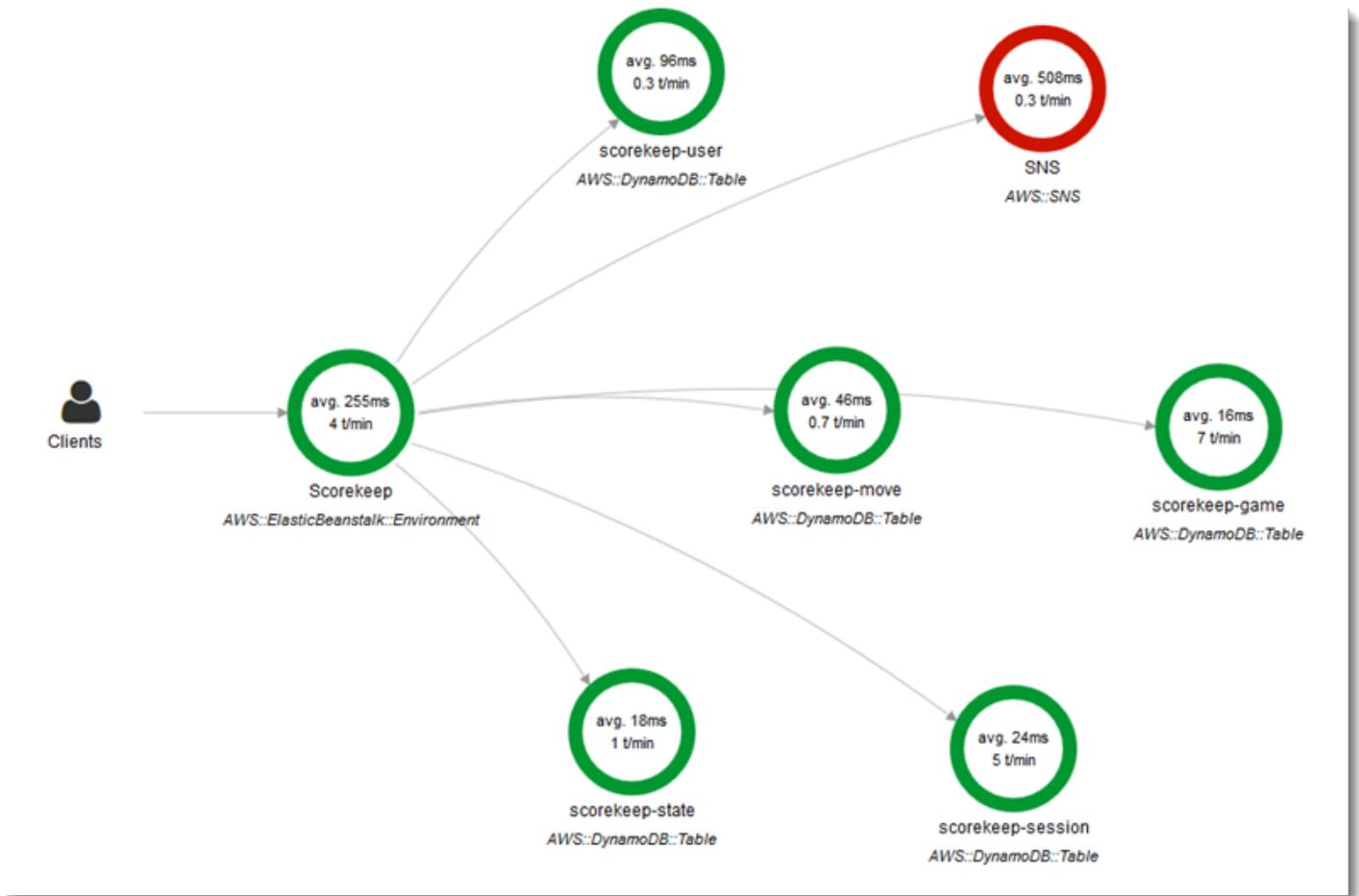
X-Ray provides an SDK that you can use to instrument your application code, and a daemon application that relays debugging information from the SDK to the X-Ray API.
