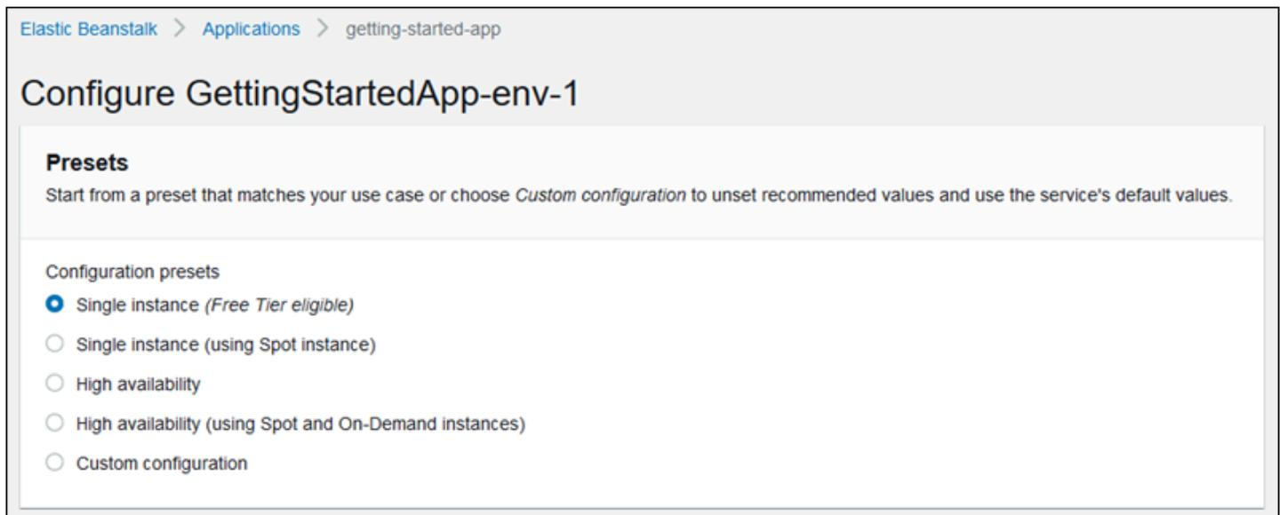
The **High availability** presets include a load balancer, and are recommended for production environments. Choose them if you want an environment that can run multiple instances for high availability and scale in response to load. The **Single instance** presets are primarily recommended for development. Two of the presets enable Spot Instance requests. For details about Elastic Beanstalk capacity configuration, see [Auto Scaling group](#).
