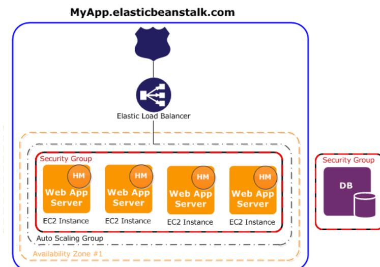
The environment is the heart of the application. In the diagram, the environment is shown within the top-level solid line. When you create an environment, Elastic Beanstalk provisions the resources required to run your application. AWS resources created for an environment include one elastic load balancer (ELB in the diagram), an Auto Scaling group, and one or more Amazon Elastic Compute Cloud (Amazon EC2) instances.
