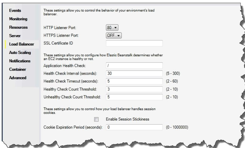
The screenshot shows the configuration window for Elastic Load Balancing in the AWS Toolkit for Visual Studio. The window is divided into a left sidebar with navigation tabs and a main configuration area. The 'Load Balancer' tab is selected in the sidebar. The main area contains the following settings:
