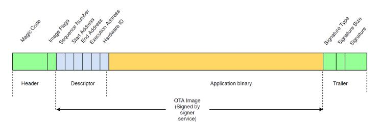
The diagram shows the primary components of the application image stored on each bank of the device.
