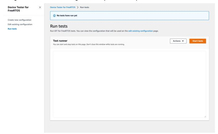
IDT for FreeRTOS runs the qualification tests. It then displays the test run summary and any errors in the **Test runner** console. After the test run is complete, you can view the test results and logs from the following locations:
