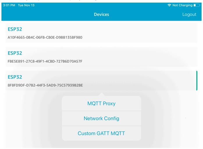
After you enable the MQTT proxy, MQTT messages appear on the thing-name/example/ topic1 topic, and data is printed to the UART terminal.
