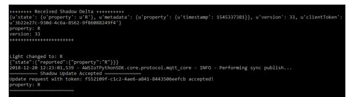
When executed for the first time, each client device script runs the AWS IoT Greengrass discovery service to connect to the AWS IoT Greengrass core (through the internet). After a client device has discovered and successfully connected to the AWS IoT Greengrass core, future operations can be executed locally.
