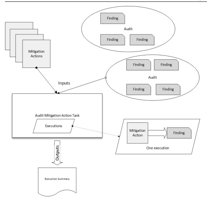
The following diagram shows how you can define an audit mitigation task that takes a list of individual findings from one or more audits and applies a set of actions to those findings. A single execution applies one action to one finding. The audit mitigation actions task outputs an execution summary.
