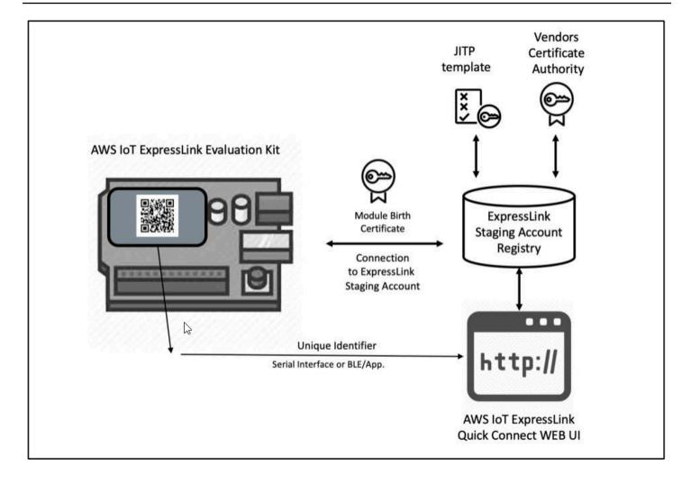
Figure 5 - ExpressLink Evaluation Kit Quick Connect flow
