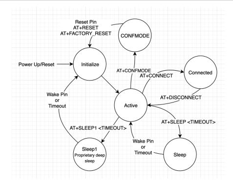
Figure 2 - ExpressLink internal states diagram (partial)
