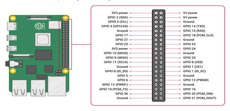
Figure 7 - RaspberryPi 4 I/O connections
