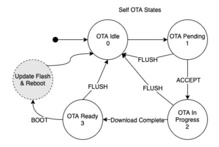
Figure 3 - ExpressLink module OTA state diagram
