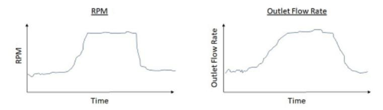
These graphs show the expected relationship between RPM and flow rate: as the pump rotates faster, the fluid flows faster. The graphs show two operating modes: one with low RPM and a low flow rate, and a second mode with high RPM and high flow rate. In this case, Amazon Lookout for Equipment wants to learn this normal relationship in terms of operating modes. The following graph shows another way to visualize the learned normal operating modes.
