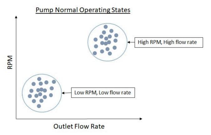
The normal behavior of this pump is clear. The operator runs the pump at low RPM and high RPM in order to get a low flow rate or a high flow rate. As the pump continues to run, we expect that the
