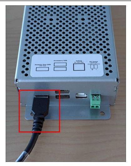
4. For POE++ power, plug in the Ethernet cable from the POE++ source into the I/O hub port.
