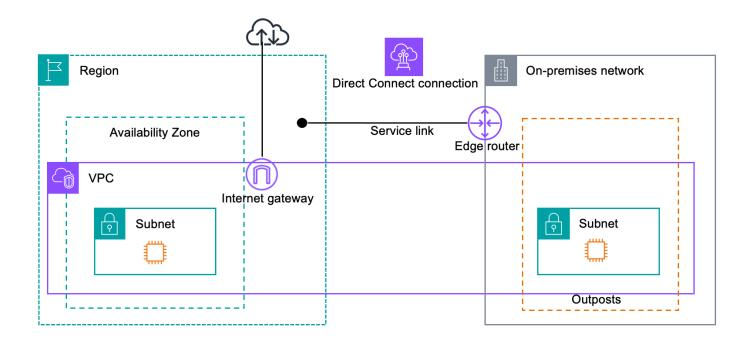
If you are using a stateful firewall with your internet connection to limit connectivity from the public internet to the service link VLAN, you can block all inbound connections that initiate from the internet. This is because the service link VPN initiates only from the Outpost to the Region, not from the Region to the Outpost.
