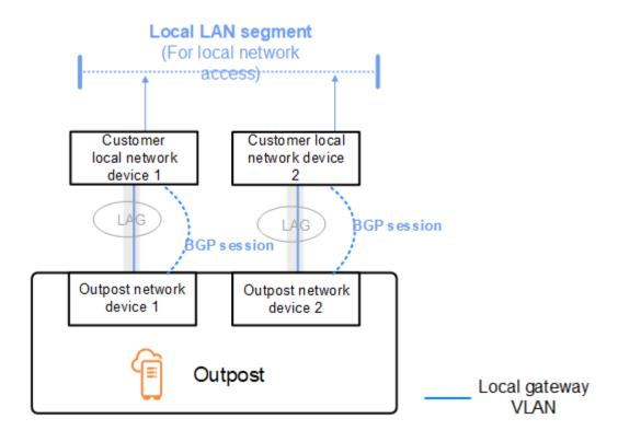
We recommend that you configure customer network equipment to receive BGP advertisements from Outposts without changing the BGP attributes, and enable BGP multipath/load balancing to achieve optimal inbound traffic flows. AS-Path prepending is used for local gateway prefixes to shift traffic away from ONDs if maintenance is required. The customer network should prefer routes from Outposts with an AS-Path length of 1 over routes with an AS-Path length of 4.
