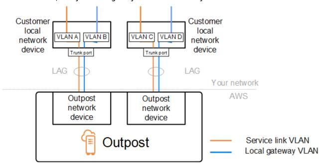
To integrate your Outpost with your on-premises network during the installation and ongoing operation, you must allocate the VLANs used between the Outpost network devices and
