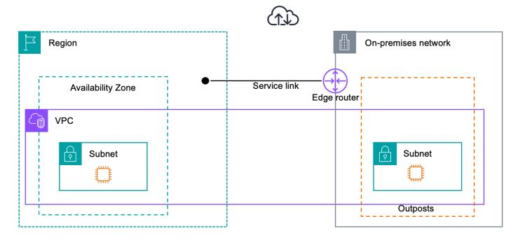
If you use a firewall to limit the connectivity from the service link VLAN, you can block all inbound connections. You must allow outbound connections back to the Outpost from the AWS Region as
