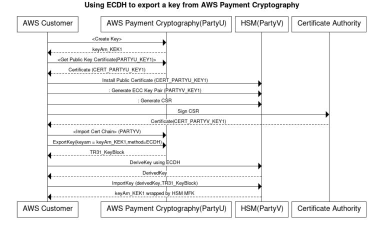
Elliptic Curve Diffie-Hellman (ECDH) uses ECC asymmetric cryptography to establish a shared key between two parties without requiring pre-exchanged keys. ECDH keys are ephemeral, so AWS Payment Cryptography does not store them. In this process, a one-time <u>KBPK/KEK</u> is derived using ECDH. That derived key is immediately used to wrap the key you want to transfer, which could be another KBPK, a BDK, an IPEK key, or other key types.
