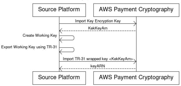
When exchanging multiple keys or supporting key rotation, partners typically first exchange an initial key encryption key (KEK). You can do this using techniques such as paper key components or, for AWS Payment Cryptography, using <u>TR-34</u>.
