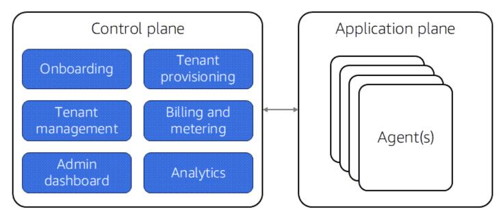
This diagram shows the traditional separation of control and application planes. What's new is that the control plane now manages the agents that make up an AaaS environment. The control plane interacts with all agents because we presume that the agents are built, managed, and deployed by one provider.
