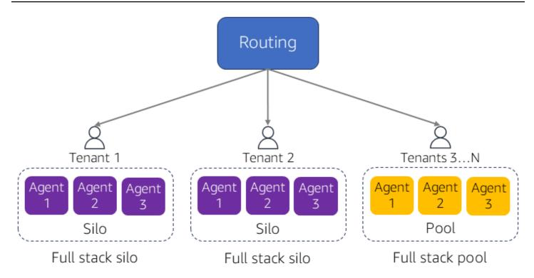
In this diagram, an agent provider has three agents that are deployed through agent as a service (AaaS). They support two types of tenants. On the left-hand side, two tenants have compliance and performance requirements that they address through a full-stack silo model. The remaining tenant on the right-hand side runs in a pooled model where tenants share resources.
