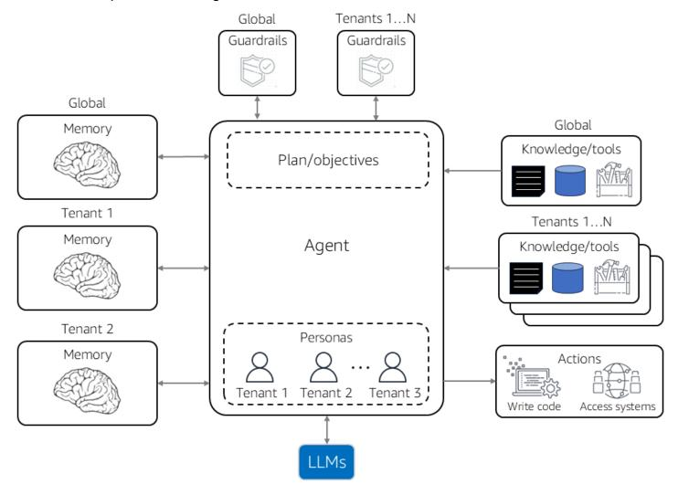
In this diagram, we introduce tenant personas that are intended to shape how an agent integrates tenant context. For example, on the left-hand side of the diagram, agent memory is altered to support tenant-specific memory. The same is true on the right-hand side of the diagram where
