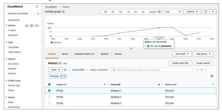
When the metric is available in the CloudWatch repository, you can display and analyze it in CloudWatch dashboards, apply further math and query operations, and set an alarm to monitor this specific metric and generate alerts if the observed values are not in line with the defined alarm conditions.
