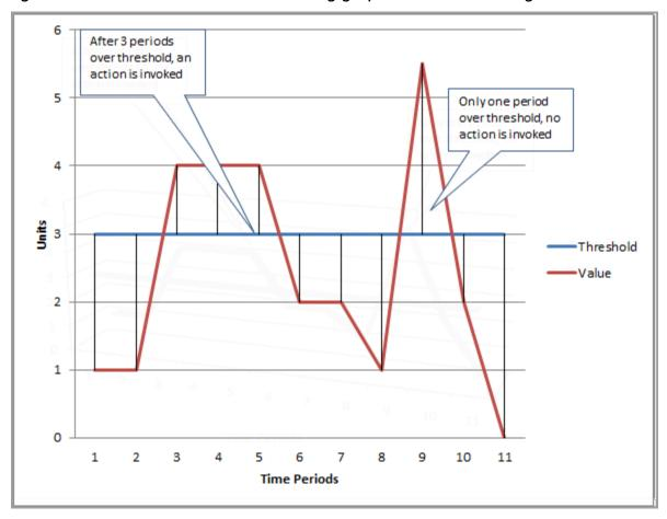
CloudWatch alarms support metric and composite alarms.
