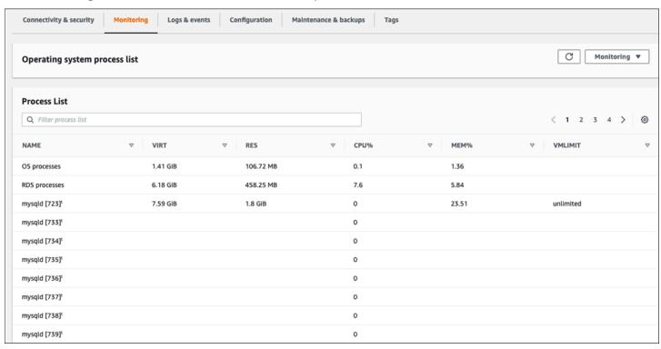
Amazon RDS delivers the metrics from Enhanced Monitoring into your CloudWatch Logs account. The monitoring data that is shown on the Amazon RDS console is retrieved from CloudWatch Logs. You can also retrieve the metrics for a DB instance as a log stream from CloudWatch Logs. These metrics are stored in JSON format. You can consume the Enhanced Monitoring JSON output from CloudWatch Logs in a monitoring system of your choice.
