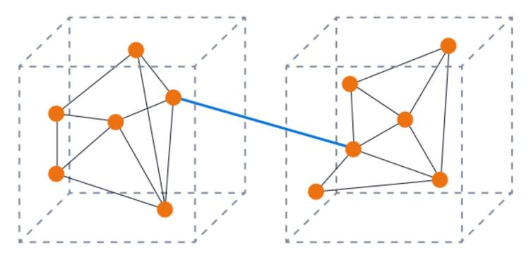
The following image shows high coupling with low cohesion. The database components are disconnected, and changes are highly likely to impact other components.
