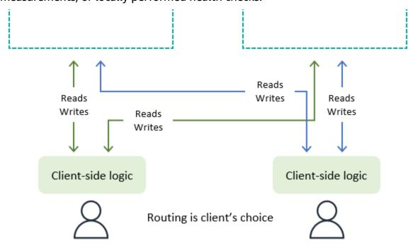
As an advantage, client-driven request routing can adapt to things such as real-world public internet traffic conditions to switch Regions if it notices any degraded performance. The client must be aware of all potential endpoints, but launching a new Regional endpoint is not a frequent occurrence.
