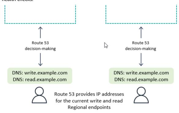
With write to any Region mode, or if combined with the compute-layer request routing on the backend, Route 53 can be given full freedom to return the Region based on any complex internal rules, such as choosing the Region in the closest network or geographic proximity, or any other choice.
