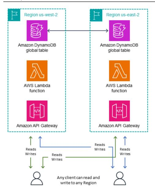
The write to any Region mode is the most straightforward architecture to implement. Routing is easier because any Region can be the write target at any time. Failover is easier, because with MRSC tables the items are always synchronized, and with MREC tables any recent write operations can be replayed any number of times to any secondary Region. Where possible, you should design for this write mode.
