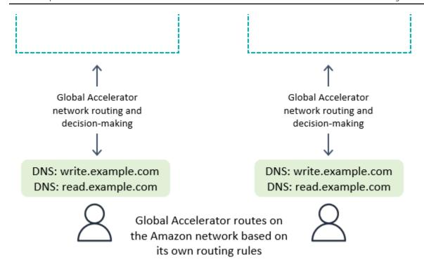
With write to any Region mode, or if combined with the compute-layer request routing on the backend, Global Accelerator works seamlessly. The client connects to the nearest edge location and doesn't have to be concerned about which Region receives the request.
