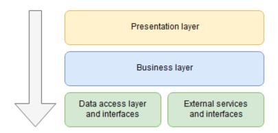
The main disadvantage of this configuration is the dependency structure. For example, if the model for storing data in the database changes, this affects the data access interface. Any change to the data model also affects the business layer, which has a dependency on the data access interface. As a result, software engineers cannot make any infrastructure changes without affecting the domain logic. This, in turn, increases the likelihood of regression bugs.
