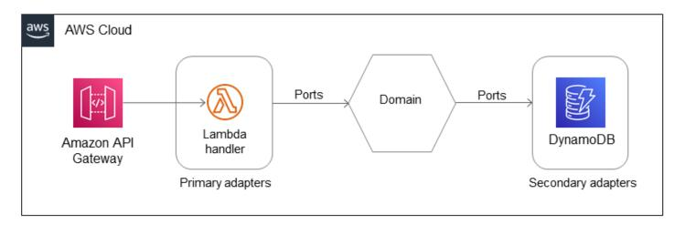
This architecture is fully serverless and gives the architect a good starting point. We recommend that you use the command pattern in the domain because it makes the code easier to maintain, and it adapts to new business and non-functional requirements. This architecture could be sufficient for building simple microservices with a few operations.
