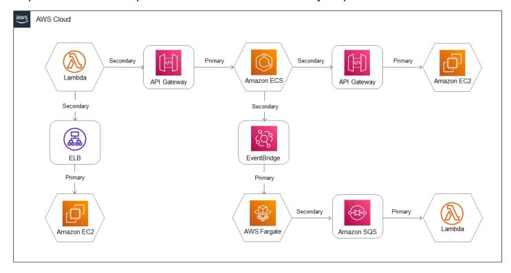
In this architecture, each domain uses a different set of compute environment(s). (Each domain might also have multiple compute environments, as in the previous example.) Each domain defines its required interfaces to communicate with other domains through ports. Ports are implemented
