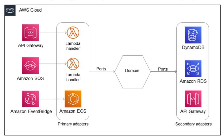
This example uses Amazon ECS as the primary adapter for launching long-running tasks in the domain. Amazon EventBridge (client) initiates an Amazon ECS task (entry point) when a specific
