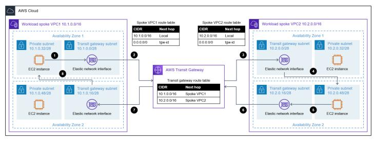
The diagram shows the traffic flow when a source Amazon Elastic Compute Cloud (Amazon EC2) instance in Workload spoke VPC 1 in Availability Zone 1 sends traffic through Transit Gateway to a destination EC2 instance in Workload spoke VPC2 in Availability Zone 2:
