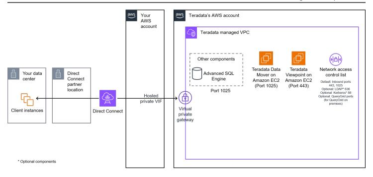
To build an architecture based on the preceding diagram, you must create a hosted private VIF and share the VIF with Teradata VantageCloud Enterprise to establish connectivity. A private VIF is a network interface that enables you to use Direct Connect to connect with another AWS account, such as a Teradata VantageCloud Enterprise AWS account. Network egress fees apply on private VIFs.
