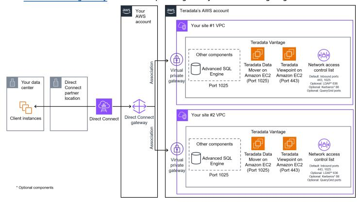
To build an architecture based on the preceding diagram, you must create a Direct Connect gateway in your AWS account and shut down the private virtual interface (VIF) to the Direct Connect gateway. You will then need to accept the association proposal for the virtual private gateway on the Teradata AWS account.
