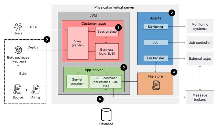
The following diagram shows the architecture of a containerized Java EE application.
