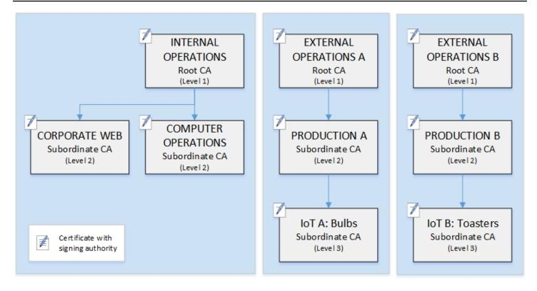
This hierarchy contains three roots, one for Internal Operations and two for External Operations (one root CA for each product line). It also illustrates multiple certification path length, with two levels of CA for Internal Operations and three levels for External Operations.
