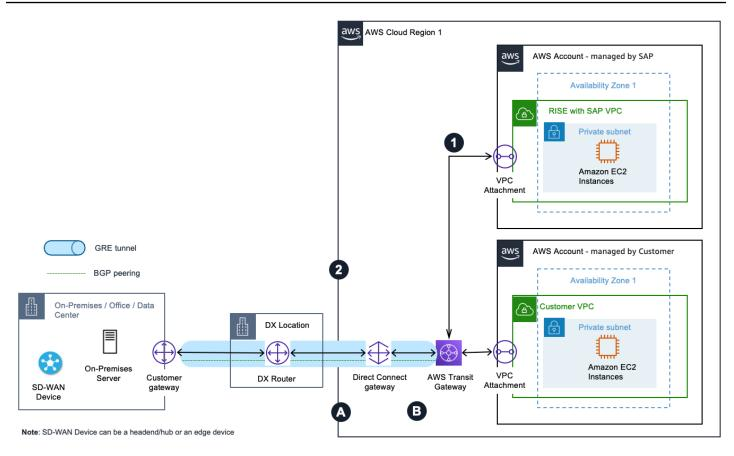
The preceding diagram illustrates a pattern of how you can extend and segment your SD-WAN traffic to AWS without adding extra infrastructure. You can create Transit Gateway connect attachments using an AWS Direct Connect connection as underlying transport in your AWS account.
