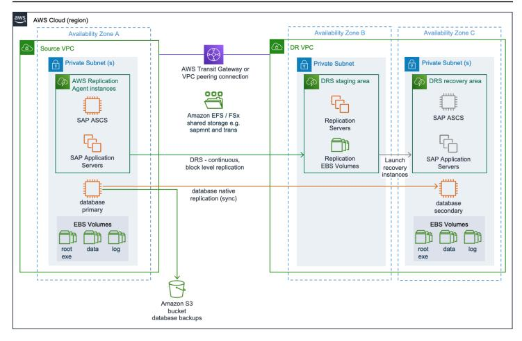
In hybrid in-Region disaster recovery implementation, the source servers running SAP application components, such as central services instance [(A)SCS], primary application server (PAS), and additional application server (AAS) are replicated using Elastic Disaster Recovery. The database is replicated using a database native replication method.
