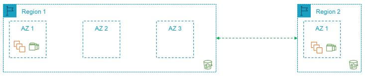
AWS isolates facilities geographically in Regions and Availability Zones. A Multi-AZ approach provides distance while maintaining performance for the primary compute capacity. This approach (Figure 5) greatly reduces the risk of location failure.
