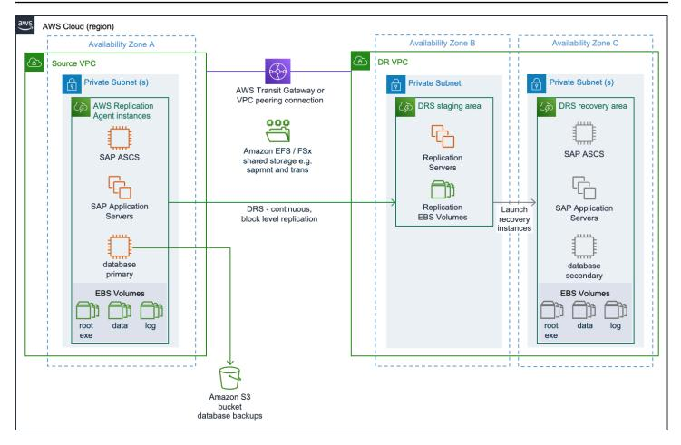
In full in-Region disaster recovery implementation, the source servers running SAP application components, such as central services instance ((A)SCS), primary application server (PAS), additional application server (AAS), and the database, are replicated using Elastic Disaster Recovery.
