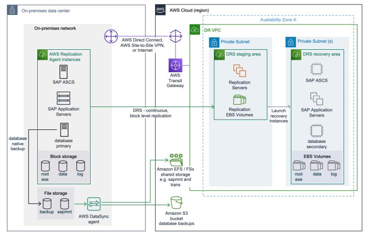
In full non-AWS to AWS disaster recovery implementation, the source servers running SAP application components, such as central services instance ((A)SCS), primary application server (PAS), additional application server (AAS), and the database, are replicated using Elastic Disaster Recovery.
