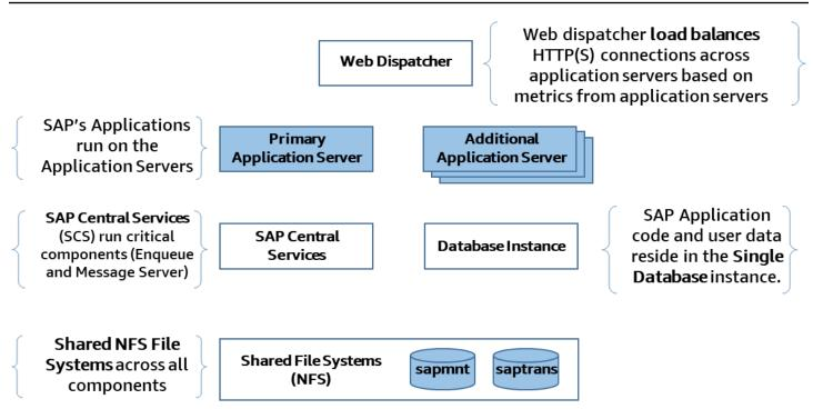
Figure 1 shows the typical SAP NetWeaver architecture, which has several single points of failure which are listed below:
