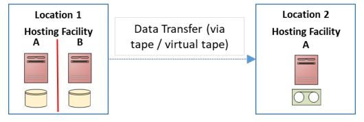
In Figure 3, we give an example of an approach that customers often take on premises. In **Location 1**, the customer has two hosting facilities often separate rooms or halls in the same data center where they deploy a high availability architecture for the SAP single point of failure. **Location 2** is the disaster recovery location in which the SAP systems are recovered, in the event of a significant failure of both hosting facilities in **Location 1**.
