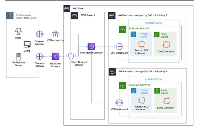
The preceding diagram displays how Transit Gateway can be used to connect multiple RISE with SAP VPCs and provide chargeback capability through the Flow Logs.
