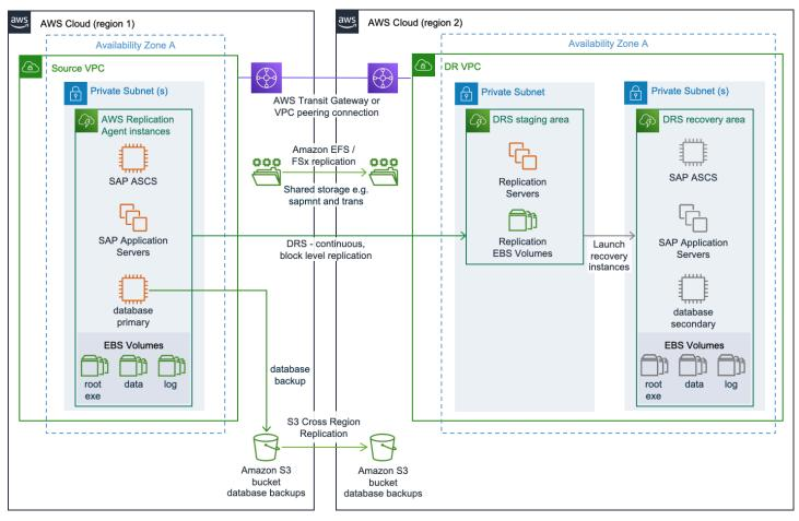
In full cross-Region disaster recovery implementation, the source servers running SAP application components, such as central services instance ((A)SCS), primary application server (PAS), additional application server (AAS), and the database, are replicated using Elastic Disaster Recovery.
