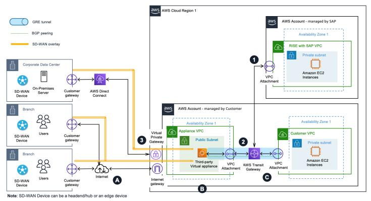
The preceding diagram illustrates a pattern of integrating your SD-WAN network with Transit Gateway using <u>connect attachments</u> and placing (third-party) virtual appliances of the SD-WAN network in an Appliance VPC within aws. It's common to have SD-WAN edge appliances deployed at branch locations, and on-premises data center to create a full mesh topology.
