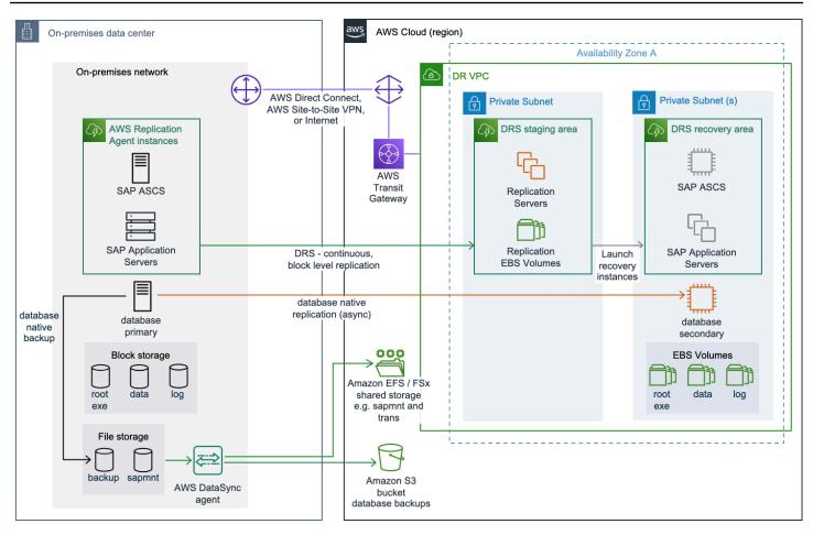
In hybrid non-AWS to AWS disaster recovery implementation, the source servers running SAP application components, such as central services instance [(A)SCS], primary application server (PAS), and additional application server (AAS) are replicated using Elastic Disaster Recovery. The database is replicated using a database native replication method.
