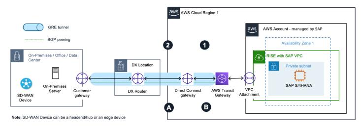
The preceding diagram illustrates a pattern of how you can extend and segment your SD-WAN traffic to AWS without adding extra infrastructure. In RISE with SAP, you can request SAP to create Transit Gateway connect attachments using a Direct Connect connection as underlying transport. Customers can leverage SAP-managed <u>Direct Connect gateway (DXGW)</u> if required.
