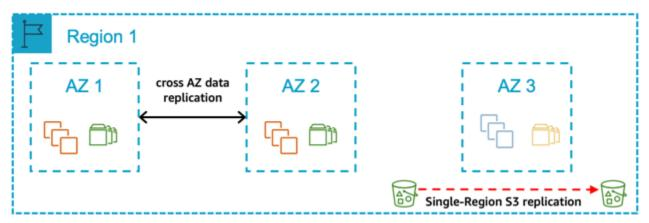
In this pattern, you deploy all your production systems across two Availability Zones. The compute deployed for the production SAP database and central services tiers are the same size in both Availability Zones, with automated fail over in the event of a zone failure. The compute required for the SAP application tier is split 50/50 between two Availability Zones. Your non-production
