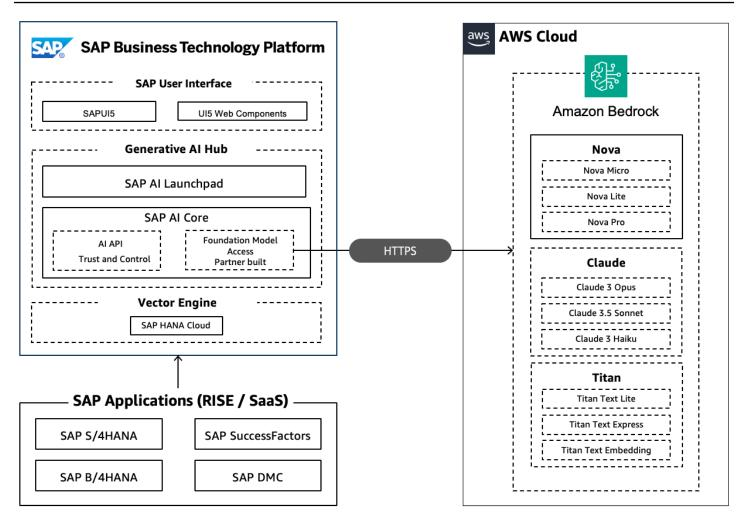
The diagram illustrates a design framework for a Generative AI solution or an S/4 HANA extension, created and implemented on the BTP. This design illustrates smooth integration with RISE and SAP Solutions that operate on AWS. utilizing the connectivity service and leveraging Bedrock LLM models through the Generative AI Hub.
