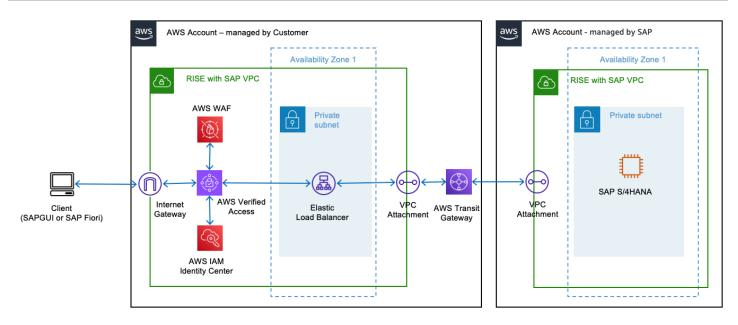
The preceding diagram describes on how AWS verified Access deployed and integrated with RISE with SAP
