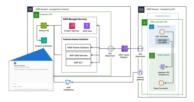
The diagram above illustrates a design framework for Q Business based search for RISE customers. It illustrates how SAP data can be extracted utilizing AWS services and using pre-built connectors from Q Business organizations can create a unified search experience.
