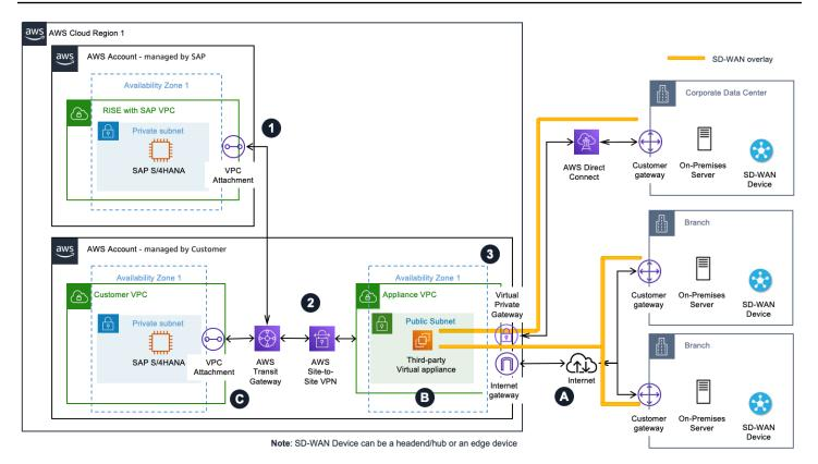
The diagram above illustrates a pattern of integrating your SD-WAN network with Transit Gateway using an AWS Site-Site VPN connection and placing (third party) virtual appliances of the SD-WAN network in an Appliance VPC within aws. You may use this option when your third-party virtual appliance does not support GRE. It's common to have SD-WAN edge appliances deployed at branch locations, and on-premises data center to create a full mesh topology.
