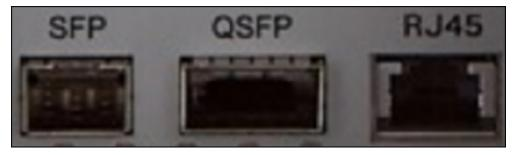
Only one network interface on the AWS Snowball Edge device can be used at a time. Hence use any one of the ports to support the following network hardware.
