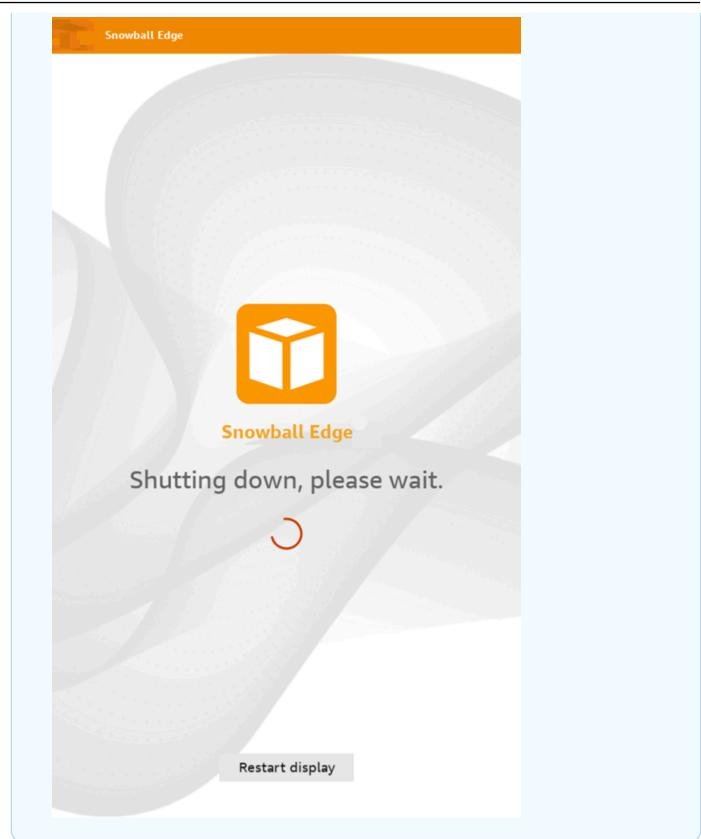
2. Press the power button. When the device is ready, the LCD display shows a short video while the device is getting ready to start. After about 10 minutes, the device is ready to be unlocked.
