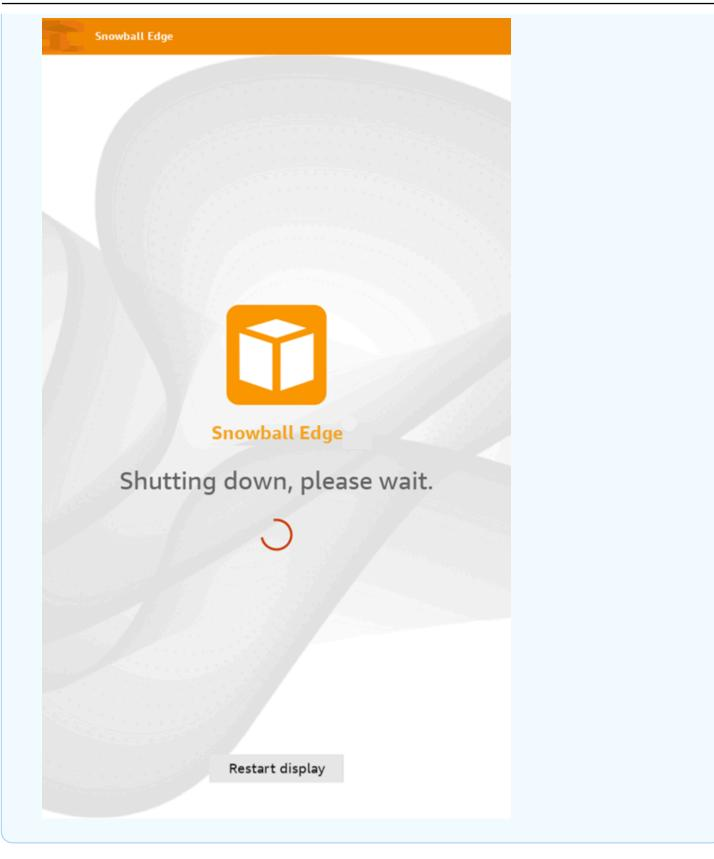
After the device shuts down, the shipping information appears on the E Ink display. If return shipping information does not appear on the E Ink display, contact Support.
