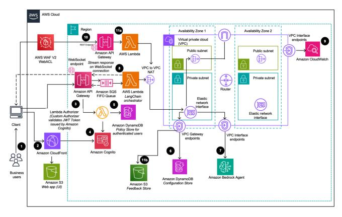
The high-level process flow for the solution components deployed with the AWS CloudFormation template is as follows:
