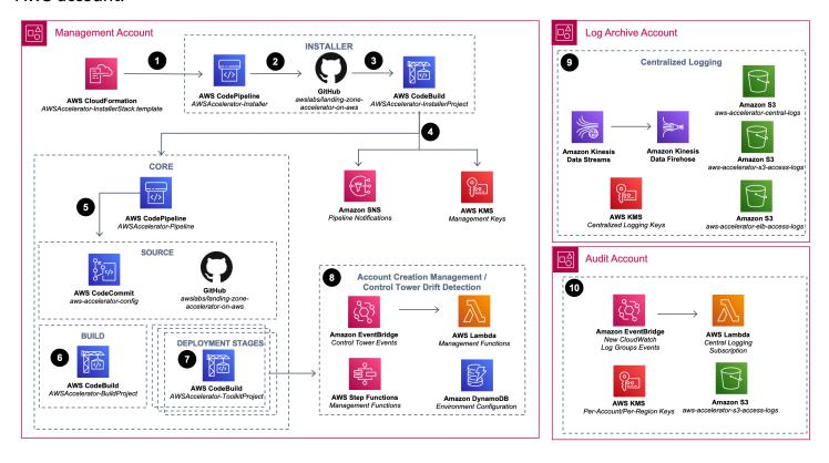
Landing Zone Accelerator on AWS high-level architecture – default resources deployed with the solution
