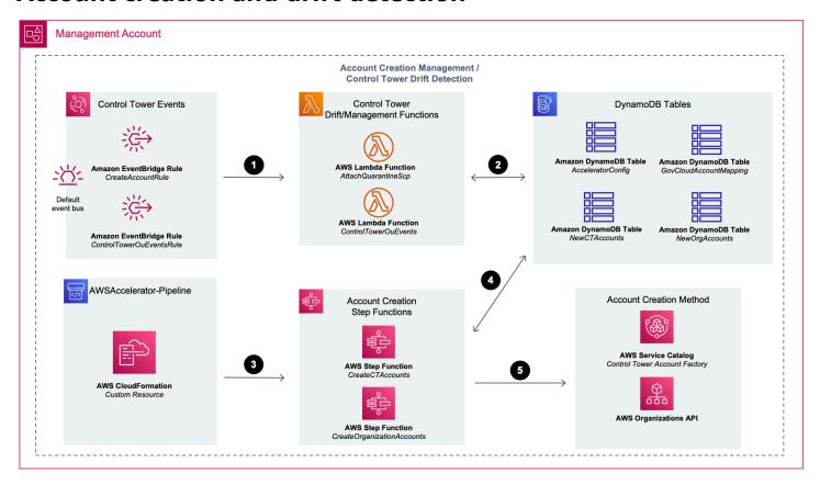
Landing Zone Accelerator on AWS architecture – account provisioning and Control Tower drift detection
