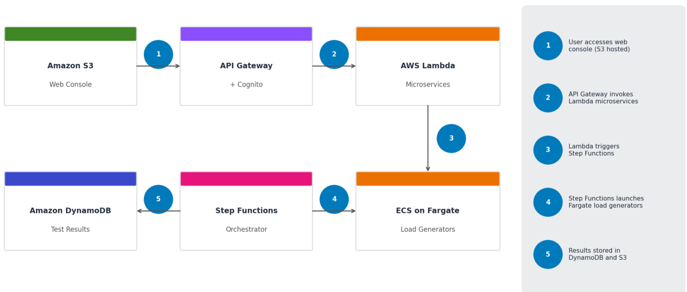
Distributed Load Testing on AWS — Architecture
