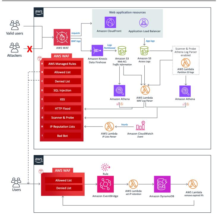
At the core of the design is an <u>AWS WAF</u> web ACL, which acts as the central inspection and decision point for all incoming requests to a web application. During initial configuration of the CloudFormation stack, the user defines which protective components to activate. Each component operates independently and adds different rules to the web ACL.
