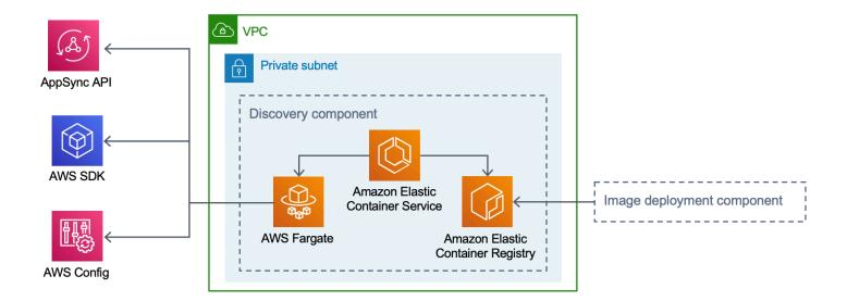
This solution configures Amazon ECS to run an AWS Fargate task using the container image downloaded from Amazon ECR. The AWS Fargate task is scheduled to run at 15-minute intervals. The resource relationship data that is collected is inserted into an Amazon Neptune graph database and Amazon OpenSearch Service.
