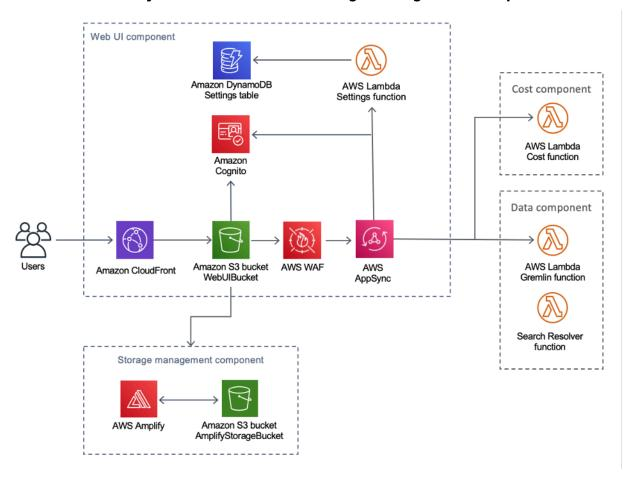
The web UI resources are hosted in the WebUIBucket Amazon S3 bucket and distributed by Amazon CloudFront. AWS Amplify provides an abstraction layer to simplify the integrations to AWS AppSync and Amazon S3.
