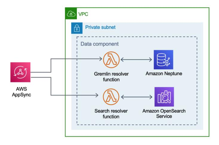
The web UI sends requests to the AppSync API, which invokes either the Gremlin Resolver or Search Resolver Lambda functions. These functions process the requests and query Amazon Neptune or OpenSearch Service to retrieve data about the provided resources. AWS AppSync also supports requests for the estimated cost data from the AWS CUR.
