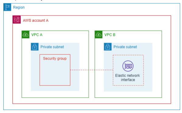
The diagram above shows AWS account A with two VPCs in it. Each of the VPCs has workloads running in a private subnet. In this case, workloads in VPC A and B subnets share the same network traffic requirements, so Account A can use the Security Group VPC associations feature to associate the security group in VPC A with VPC B. Any updates made to the associated security group are automatically applied to the traffic to workloads in the VPC B subnet.
