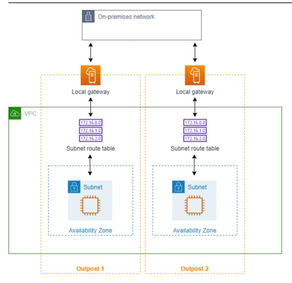
To enable this feature, add a route to your Outpost rack subnet route table that is more specific than the local route in that route table and has a target type of local gateway. The destination of the route must match the entire IPv4 block of the subnet in your VPC that is in another Outpost. Repeat this configuration for all the Outpost subnets that need to communicate.
