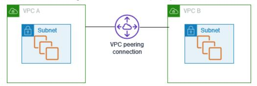
The process of creating a VPC peering connection leverages the existing VPC infrastructure to establish this connection, without the requirement of a gateway, AWS Site-to-Site VPN, or
