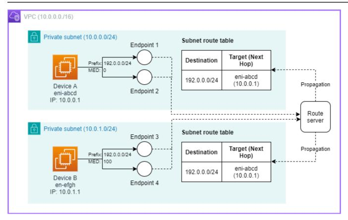
This last example below shows how route server handles failover. While the higher MED attribute tells route server that Device B is less preferred than Device A, if Device A eni-abcd (10.0.0.1) goes down, route server updates the subnet route tables, and traffic to 192.0.0.0/24 is routed to Device B eni-efgh (10.0.1.1) as the next hop.
