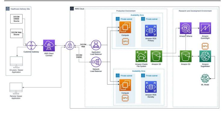
A cloud-based medical imaging system, such as a PACS or VNA, on AWS. High availability and lowlatency study retrieval for medical imaging solutions.
