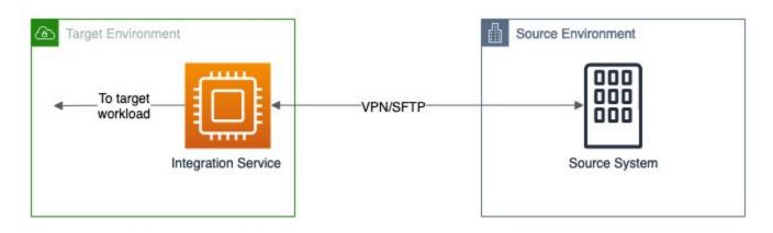
A common HL7v2 interoperability architecture where the integration may exchange HL7 v2 messages through a VPN tunnel or SFTP. MLLP over TLS can help keep messages encrypted in transit.
