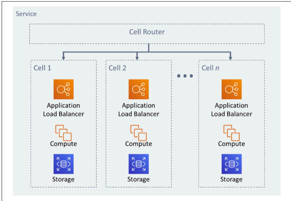
Figure 11: Cell-based architecture
