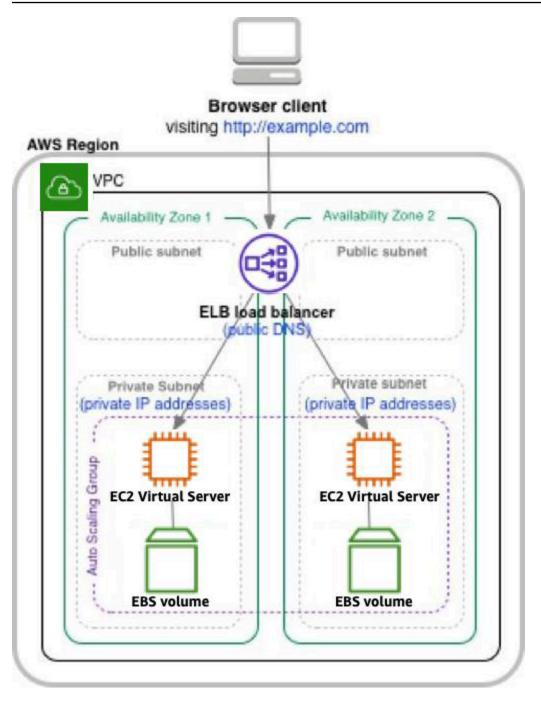
AWS architecture for a "Lift and Shift"
