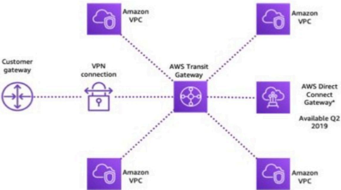
Figure 12 – Network connectivity before and after introducing AWS Transit Gateway
