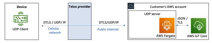
Architecture of a customer-operated solution secured by DTLS
