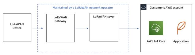
Example architecture for using a public LoRaWAN network with AWS
