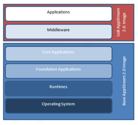
Using a base AppStream 2.0 image in Desktop View (Foundation and Core applications) with an additional AppStream 2.0 image (LoB applications) to deliver a complete set of applications
