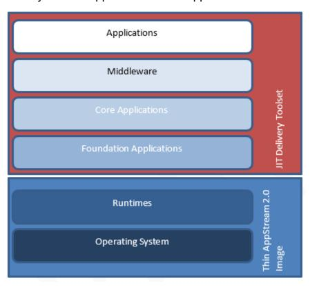
Using a thin AppStream 2.0 image and JIT delivery toolset to deliver a complete set of applications
