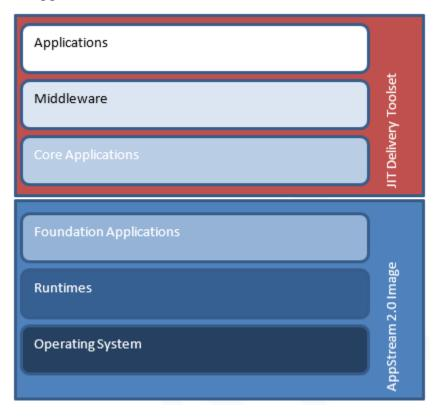
Using a baseline AppStream 2.0 image with a JIT toolset to deliver a complete set of applications
