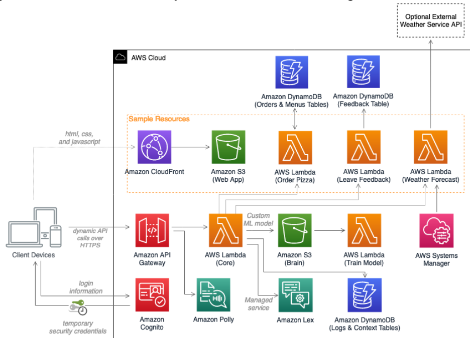
Figure 1: Serverless Bot Framework reference architecture
