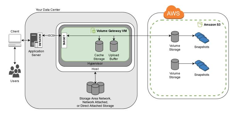
After you install the Storage Gateway software appliance—the VM—on a host in your data center and activate it, you use the AWS Management Console to provision storage volumes backed by Amazon S3. You can also provision storage volumes programmatically using the Storage Gateway API or the AWS SDK libraries. You then mount these storage volumes to your on-premises application servers as iSCSI devices.
