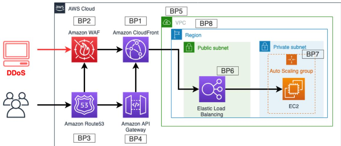
Figure 5: DDoS-resilient reference architecture
