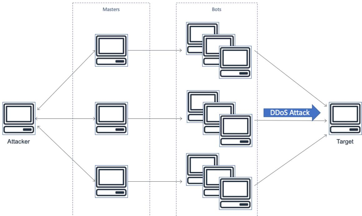
Figure 2: Diagram of DDoS Attack
