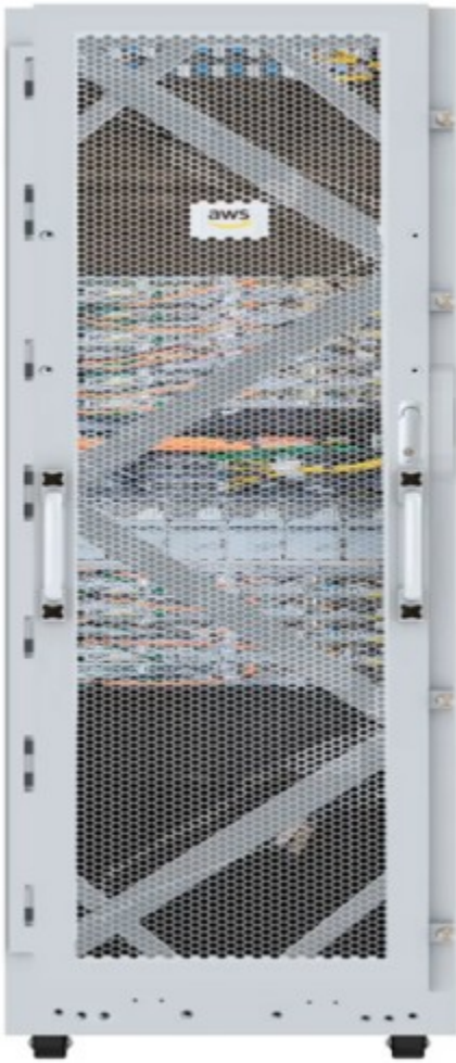
Figure 29 – AWS Outposts form factors (1U, 2U, and 42U)
